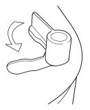
8. Lift latches up on both sides of panel to release.
